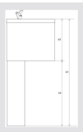
L1 = 900mm L2 = 352mm L3 = 548mm L1 = 800mm L2 = 352mm L3 = 448mm L1 = 700mm L2 = 352mm L3 = 348mm
